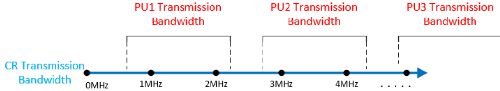
Figure 2.2: CR Transmission Interfere with Primary Transmissions
